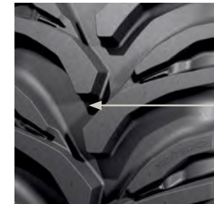
Nokian Tractor King tread depth measuring point
