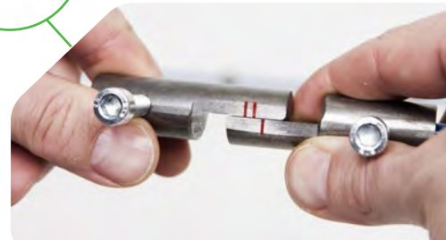
Mandrel gauge for rim circumference measurement
